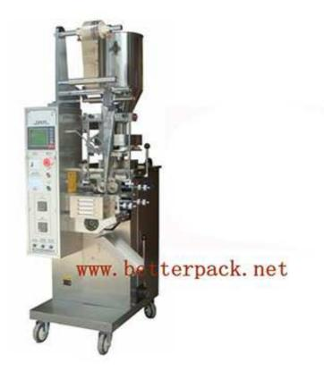
It is suitable for the package of broken tea in filter paper.
