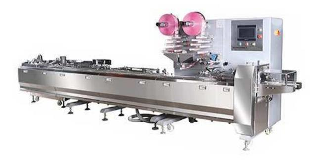
This model is used to packing cylindrical shape, unregular shape, etc, like chocolate enrobing bar, cereal bar, wafer etc.
