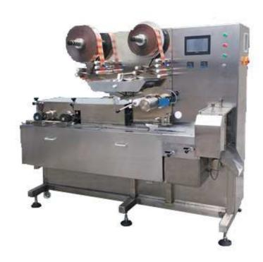
FWM500B Cut and Flow-pack is applicable to cutting and packaging chewing gum, bubble gum, soft candy or hard candy. Small compact machine which consists of two sets of vertical rope forming wheels for either round, square, oblong & flat section profile pieces. The pieces are automatically cut with nipper knives, transported along a transport conveyor as a flow-pack, giving speeds of up to 500 packs per minute.
