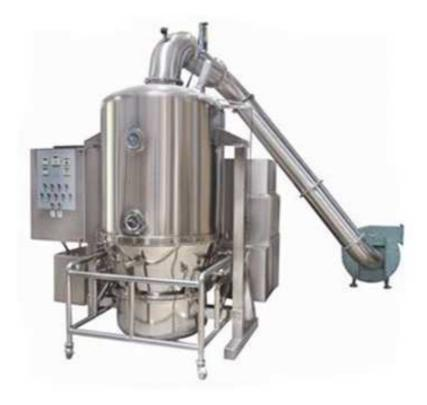
Prism Fluid Bed Processing involves fast drying, cooling and agglomeration of particulate materials. It is ideal for heat sensitive and non-heat sensitive products in Pharmaceuticals, Chemicals and Biochemical, Food and Dairy Industries.
