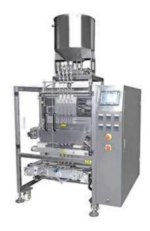
Automatically measuring, making bags, filling, sealing, cutting, printing the lot number and finished product conveying. Applicable for the liquid product, such as medicinal liquid, ice lolly, milk, water, ketchup, oil.etc.
