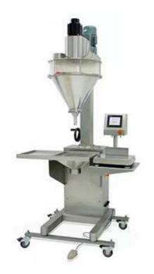
The powder packing machine is controlled by a single chip and has functions such as automatic quantitative, automatic filling, and automatic adjustment of measurement errors.
