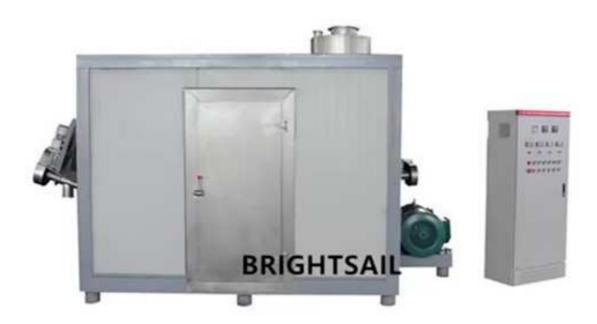
BS cryogenic grinder is one of our latest products, liquid nitrogen was used as the cryogen energy to achieve high-quality grinding of materials at low temperature. It can be used for grinding of medicines, food and plastics of the field of high value-added at low temperature.
