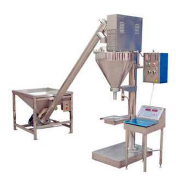
The powder filling machine is suitable for the packing of powder materials in the chemical, food, agricultural industries; such as: milk powder, rice flour, corn starch, chili powder, coffee powder, washing powder, seasonings, feed etc.
