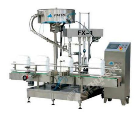
The machine used straight bottle feeding and control by PLC program. Bottles will be fixed by two cylinders and it can automatically arrange lid, taking lid and sending lid, it will first grasp lid then capping under control of double-acting cylinder lifting stroke. The machine grasp lids through pneumatic type, lid-revolving head has a clutch to ensure the tightened lid not to damage. It suits for capping of 5-25kg drum plastic large diameter caps.
