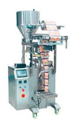
Mixing powder filler vertical packaging machine is applicable for the granule packaging and granule powder, like detergent powder, such as peanuts, walnuts, pistachios nuts, dried sea shrimp, powdered pork floss, coffee beans, seeds, rice, spice granule, peanuts, MSG, sugar, Fish Feeds, glucose, Popcorn, crispy rice, Frozen French Fries, Corn Puff / Nik Naks, spirulina cereal and etc.
