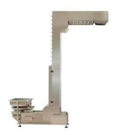
Bucket conveyor (also called Z type bucket conveyor) consists of frame, buckets, chains, sprockets, control box and other accessory are used to vertically convey bulk or loose materials efficiently. Bucket elevators can elevate a variety of bulk materials from light to heavy and from loose, flowing fine materials to larger, partially fragile objects.
