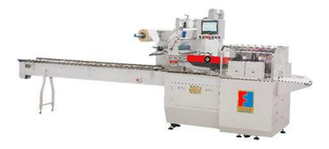
FFA-SM is specialized on the pharmaceutical industry of infusion and tablets which requires high moisture proof, thicker packing film (60-120microns), and high packing speed. This reciprocating type packing machine adopts two synchronous cutters. In the same rpm, the two cutters cut and seal the package synchronously, one packet in one process circle, this will greatly improve the production efficiency.
