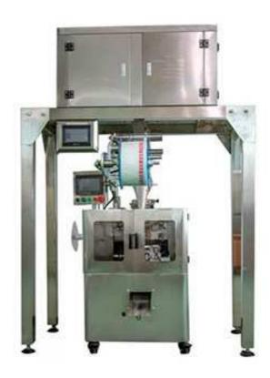
MODEL: XH-SJB is an independent Naked Pyramid Tea Bag Packing Machine. It uses the mesh bag film roll which is made of PLA/nonwovens/nylon as the packing material. Flat packages and triangular packages can be switched for your needs. It is widely applied to various regular and irregular materials like loose tea leaf, Whole leaf tea, blend tea, herbal tea, and fruit tea, etc.
