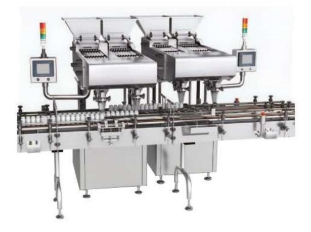
Fully automatic bottle filings machine, max speed is up to 100~200bottle/min
