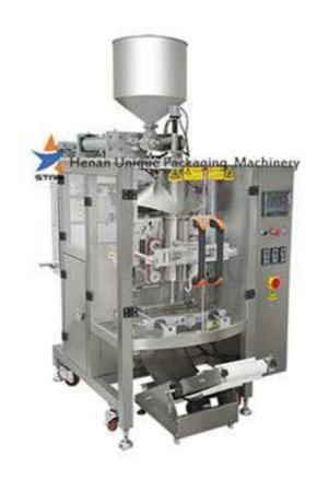
Mustard Oil Automatic Packaging Machine adopts PLC computer control system, and the operation is more stable, can adjust any parameters without stopping. The servo motor is used for pulling and the positioning is more accurate.
