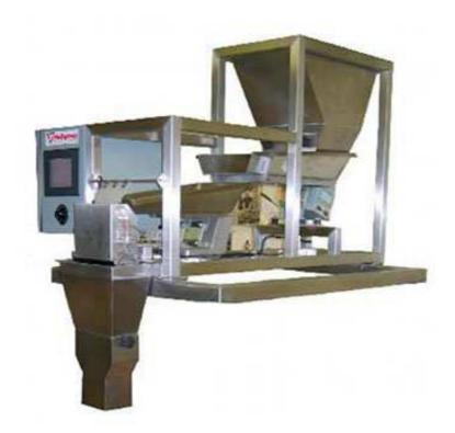
The Tridyne F-100 Series of Net Weigh Fillers are available in 4 different configurations. It can be used as a table top model or can be integrated with other industrial bulk filling equipment such as baggers, conveyors, sealers, and more. Products need to be free flowing.
