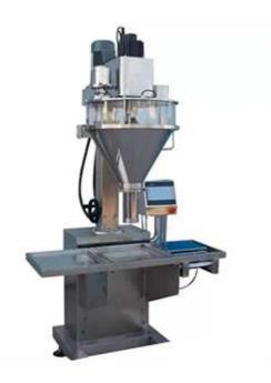
Semi-automatic powder filling machine touch screen operation, simple and easy to operate, suitable for filling food, chemical powder and granular products.it fits more to the fluidic or low-fluidity materials, like milk powder, albumen powder, pharmaceuticals, condiment, solid drink, white sugar, dextrose, coffee, agriculture pesticide, granular additive, and so on.
