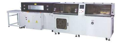
This machine uses PLC, colorful touch screen and servo control system and greatly improves the accuracy of speed adjusting, bag forming and length cutting, so the machine is running with high reliability and supreme performance, easy and convenient to operate.
