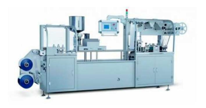
DHC-250P is a multi-functional automatic blistering machine. The machine can automatically form, detect empty blisters, feed product, detect product, press, strike and cut blisters. Strokes can be adjusted with servo motor driver control.
