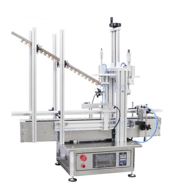
The desktop capping machine is suitable for different sizes of bottle caps, the capping chuck can be customized according to your need, you can customize several pieces of capping chuck for multiple sizes of bottles. This one is with the cap feeder which can make it possible to feed caps faster.it can work automatically and help you save labor and time, help you improve working efficiency.
