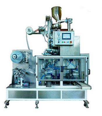
Model DXDC50I is our new pyramid (triangle) tea bag with three-side sealing flat envelope packing machine. It is used for the packing of tea leaves, such as green tea, black tea, oolong tea etc. The pyramid bags have good perviousness and perspectivity. Each pyramid tea bag is individually wrapped by envelope for freshness.
