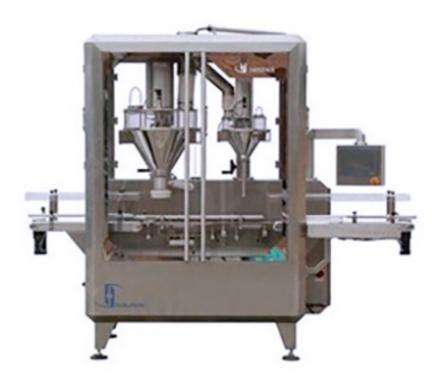
Our integral line system/powder filling line is designed for filling powder products into bottles or cans. Our staff will help you to plan and suggest you the best machine choice to use. Auger has the complete filling machine types to provide to the business owners and they can consider purchasing the machines with single unit or full integral production line.
