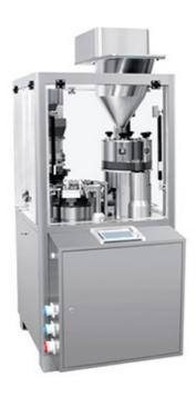
NJP-400A Fully Automatic Capsule Filling Machine is filled by powder, grain, and tablet. It adopts multi-bore dosing, intermittent motion and timing frequency conversion. It is suitable for automatically completing capsule feeding, separating, filling, (waste capsule rejecting), closing, finished product ejecting for powder or tiny pill medicine in capsule. It is designed sophisticatedly by our factory according to the practice on domestic; it is fully accord with the GMP standard.
