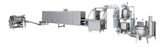
This production line can produce gelatin or pectin based jelly candy, also can produce the 3D jelly candies. The depositor also can be used to produce the deposited toffees via change-over the moulds.
