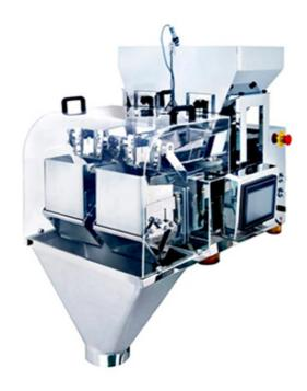
Automatic Linear Weigher Machines, also known as linear weighing machines or linear weighers are advanced devices designed to accurately measure and dispense predetermined quantities of products for packaging. These machines make use of a linear weighing mechanism where products are transported along the linear conveyor belt system and weighed at different stages before being packaged.
