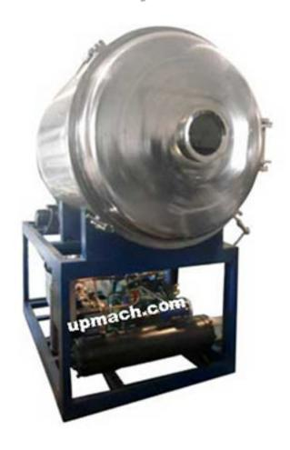
JDG food vacuum freeze dryer is used to remove a solvent (usually water) from dissolved or dispersed solids. Freeze drying is the method for preserving materials which are unstable in solution. In addition, freeze drying can be used to separate and recover volatile substances, and to purify materials. The fundamental process steps are: freezing, vacuum, heat and condensation.
