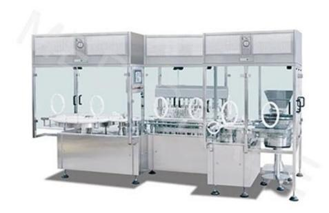
The machine is a straight line continuous or intermittent full servoing filling machine. The Cilin bottle enters the synchronous belt through the bottle plate and completes the filling and plugging of the liquid in the process of continuous or intermittent transmission, and it is sent to the downstream equipment or out of the bottle storage plate.
