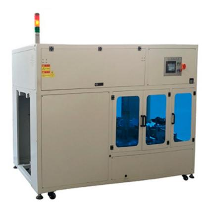
The automatic paper tray former also called Tray erector or tray packer adopts pneumatic control, which is automatically folded and formed through the mold, and the paper flap automatically locks the cardboard, so that the cardboard forming does not need to be sealed with tape or hot melt glue.
