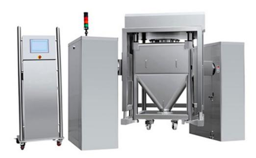
The machine can automatically complete all actions such as lifting, clamping, mixing, and lowering. Equipped with an automatic lifting hopper mixer and multiple mixing hoppers of different specifications, it can meet the mixing requirements of large quantities and multiple varieties. It is an ideal equipment for total mixing in pharmaceutical factories. At the same time, it is widely used in pharmaceutical, chemical, food and other industries
