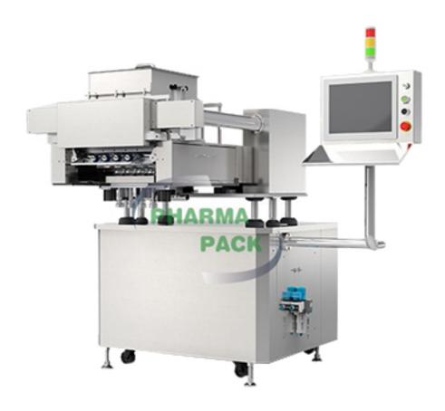
The powder filling machine is a production line specially equipped for powder filling; it is a device with online metering and filling functions.
