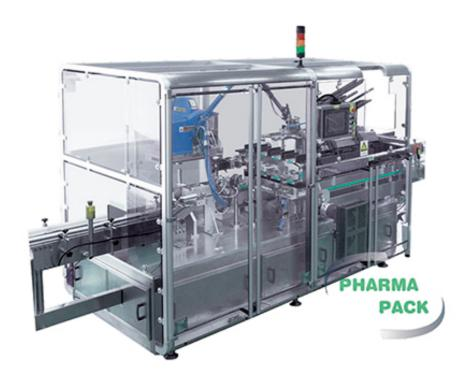
Put the bottles, carton, trays and other materials into the trays and display box packing machine in a certain arrangement and then seal the boxes.
