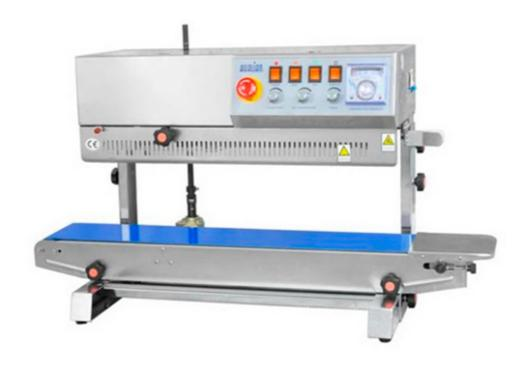
FRBM-810II is a tabletop vertical band sealer. Pre-made bags are sealed standing up, which is ideal for powder, liquid or solid products that would spill if sealed laying flat. The sealing unit can be adjusted in height to suit different sizes of packages. The FRBM-810II is equipped with PTFE seal belts and can adjust the temperature from 0 to 300°C. Equipped with solid ink coding system to achieve different color and content coding requirement.
