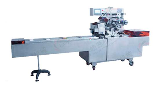
The machine adopts multi station turntable alternative packaging mode, all wrapping and heat-sealing actions are completed by cam drive, with the characteristics of fast speed and stable operation. The frequency converter is used to adjust the packing speed, which can reach 20-30 packages / min according to the different packing items. Changing the mold can pack different sizes of items.
