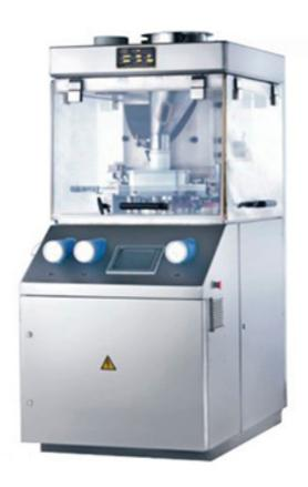
The machine is one kind of single side rotary tablet press machine which can press granular materials into round shape tablets, irregular tablets or double-side engraved tablets. This machine is mainly used in pharmaceutical, chemistry, foodstuff, electronic industries.
