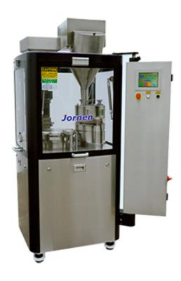
This series of Capsule filling Machines adopts a programmable control system, touch screen panel, speed-shift, and electronic automatic counter.
