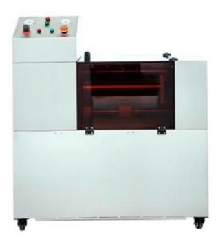
The Vacuum Decapsulator creates the air jet to transform 4-5 bar compressed air provided by outside air source into the high-frequency pulsed vacuum. The high-frequency pulsed air continuously draws capsules in the working chamber within a certain period. As a result, capsules separate gradually; powder or pellets inside fall down into the barrel. Due to flexible forces instead of mechanical forces, capsule shells keep completely intact; no fragment created in this process
