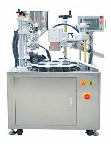
SPX-006 Ultrasonic sealing machine is advanced equipment for plastic tube sealing and aluminum plastic tube sealing. It uses ultrasonic seal the plastic tube heat shock effect produced by the transducer and to rapidly melt adhesive.
