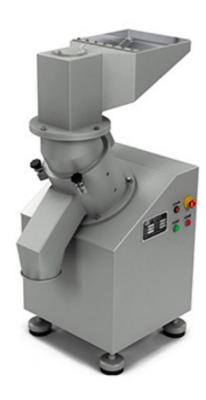
This machine is of hammer type with high speed and applied for crushing materials with medium hardness and viscosity. The material is fed into the crushing chamber through a hopper and crushed by high speed rotating hammer. The machine whose crushing chamber is easy to assemble and clean, has simple structure. Wholly made of stainless steel, the machine makes the crushed material met the hygienic requirement.
