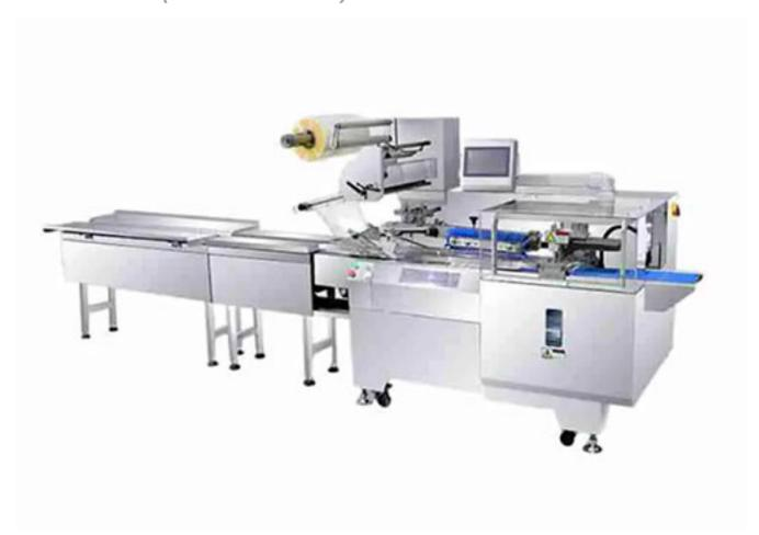
Pillow packaging machine using roll film bag-making, widely used in the packaging of various bag products; the main models are standard, wide, high-speed, back-seal, shrink film and other models.
