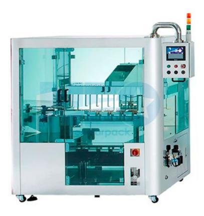
Bottle washer, 8 nozzles air wash bottle rinsing machine
