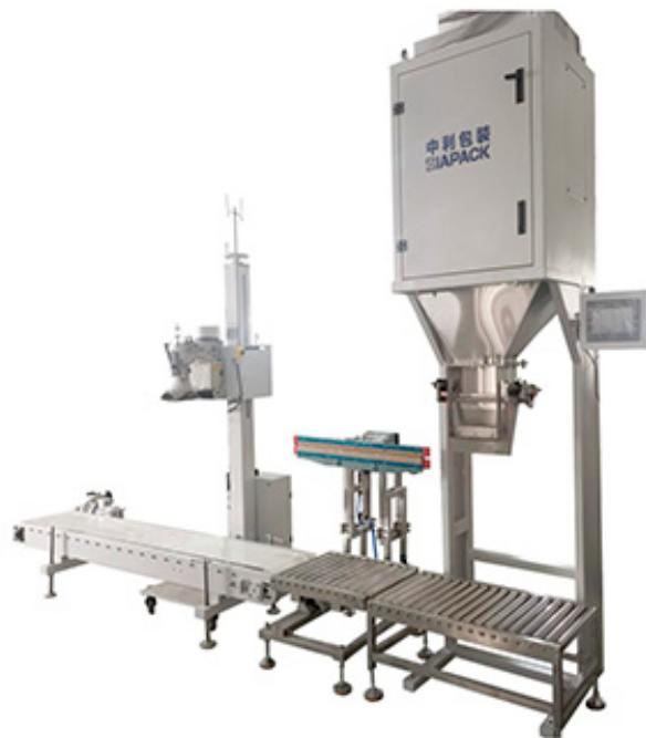
This machine unit including one set double bucket weighing machine for measuring 25-50kg. One set 3 meter output conveyor, one set pp woven bag stitching machine. The whole machine can automatic finish product weighing, product filling, automatic bag stitching and heat sealing. Just need manual feeding the bag. Widely used for semi-automatic bagging of granule product like beans, rice, plastic granule, fertilizer and so on.
