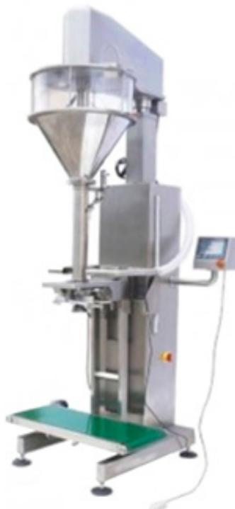
For 10~50kg semi-auto powder packing machine, we use this kind of vertical type powder filler for weighing filling. Equipped with sealing machine for plastic bag, Equipped with sewing machine for sewing.
