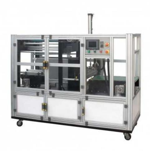
Shrink wrap machines apply heat to shrink a plastic film around a product. This process is often done by automated equipment, but manual and semi-automatic shrink wrap machines are also available. Shrink wrap machines cover the item, and then sent it through a heat tunnel or oven for shrinking.
