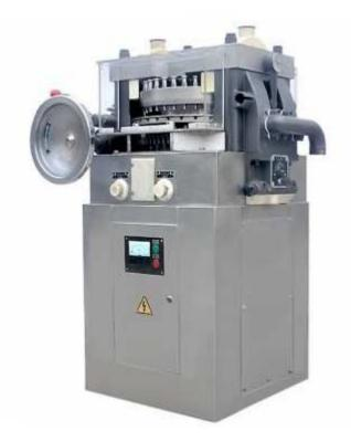
Tablet press for two-layer tablets from the company HuaMao can operate automatically and continuously producing tablets. This setting is used to produce two-layer tablets of round, sugar tablets and calcium tablets. At this point the tablet press is widely used for the manufacture of tablets in the pharmaceutical, chemical and food industries, using a powdered material as a starting substance.
