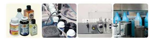
Using a synchronized swing-hand secondary alignment mechanism to ensure extra precision in the normal front/back labeling mode for oval, rectangular, and other shaped bottles. Also equipped with an added-on turn-table for stationary bottle rotation to achieve wrap-around labeling on round bottle with orientation.
