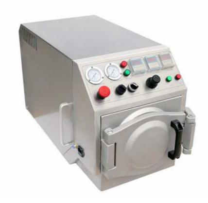
In the relatively airtight environment-working cabin, use high and low pressures to alternate changes rapidly "pressure shear" causing pulsed drawing force to the capsule. Under the continuous function of the pulsed drawing force, the capsule is gradually drawn and separated.
