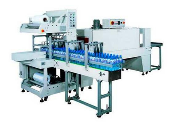
VS-6030A Automatic Shrink Packaging Machine is used for packing the beverage, beer, mineral water, pop-top cans and glass bottles with a tray or a carton etc. It is designed for the single product or the products with a tray, the sealing machine can be connected with the production line and with its auto feeding, film wrapping, sealing & cutting, shrinking and cooling, need not an operator.
