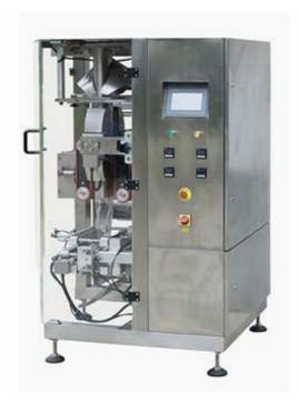
The 4-side sealing bag VFFS (Vertical Form Fill Seal) machine is suitable for packing granule, power, solid state materials, such as coffee, potato chips, puffed food, shrimp crackers, peanuts, nuts, popcorns, salt, sugar, tea, seeds, etc.
