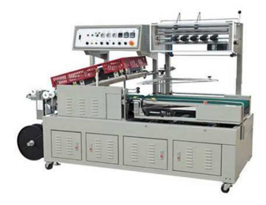
Traditional Middle speed L bar sealer has no reciprocating sealing function, so the sealing line is not strong enough and has the holes or welding seams after shrinking. The new model of TY-703-150 is designed to avoid these problems.
