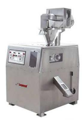
Roller compactor is used to compress fine powders into denser sheets using mechanical pressure. The basic concept of compaction is to force fine powders between two counter rotating rolls. As the volume decreases through the region of maximum pressure, the material is compressed into dense sticks or corrugated sheets.
